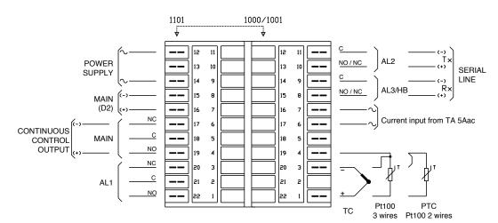
21 connections are available for 6.35 mm faston terminals. Signal inputs
